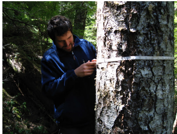
Figure 1: Tree diameters are measured by wrapping a measuring tape around the trunk of a tree 1.37 meters above the ground and then dividing the recorded circumference by \pi . Here Robert Ettinger is recording tree diameters in the Pacific Northwest. Photo :copyright: Ailene Ettinger, used with permission.
